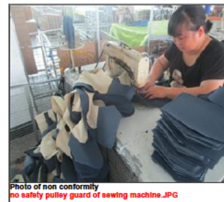
Photo of non conformity no safety pulley guard of buttoning machines.JPG
